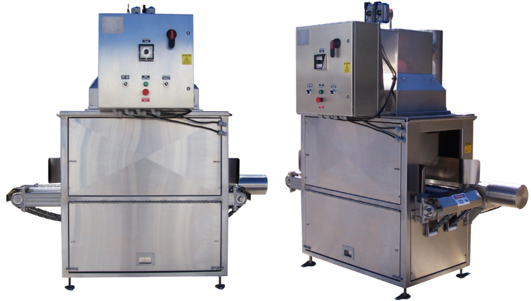
Automated Box Chilling System with exhaust hood.
