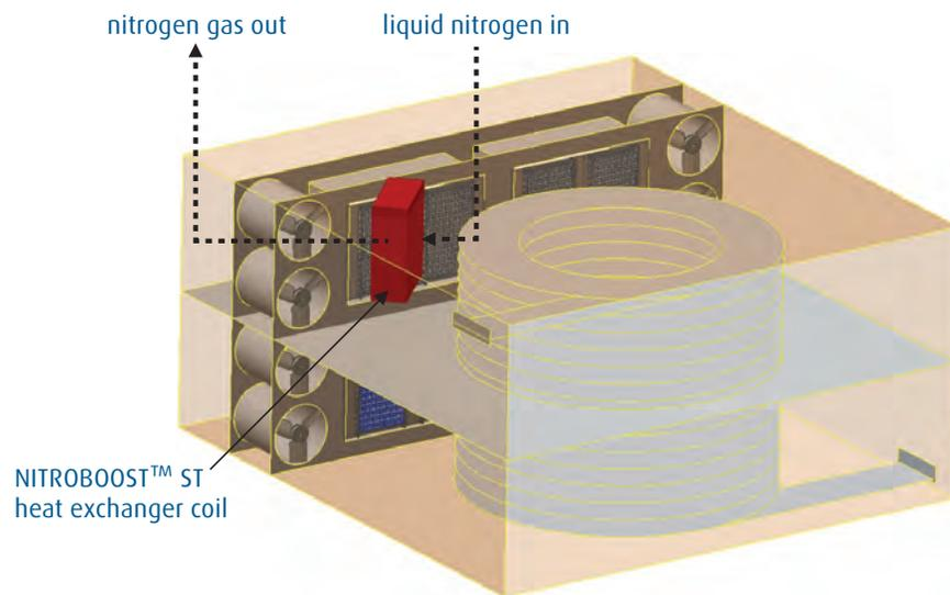
*NITROBOOST heat exchanger coils installed within spiral freezer interior.*
