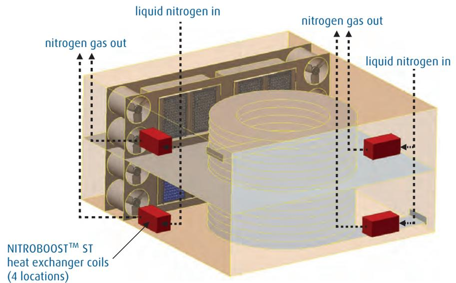
*NITROBOOST heat exchanger coils installed on spiral freezer exterior.*
