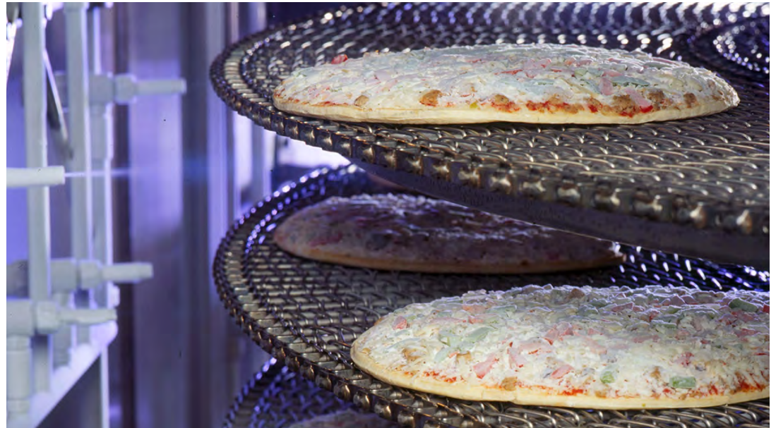
Fully assemble pizzas being frozen prior to packaging in a CRYOLINE® UPF ultra performance plus spiral freezer.
